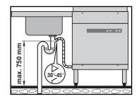
The connection between machine and site drain must not exceed the max. height of 0,75 m.
