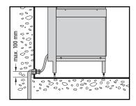
For these machine types, a floor drain is mandatory. Otherwise, residual water may remain in the tank and hose.
